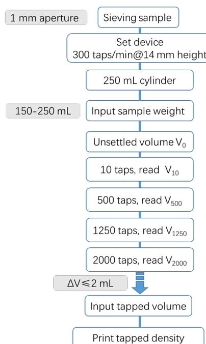
Figure 1. The test procedure
